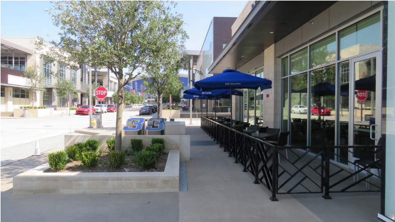
From left to right, active roadsides as a social space include an edge and furnishing zone, the throughway, and a frontage zone.
