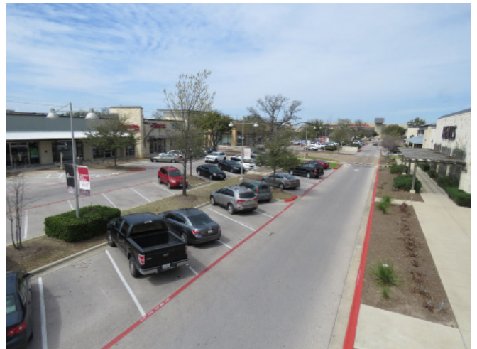
Neighborhood commercial scale should be complimentary to adjacent residential dwellings (top). Driveways within proximate large scale shopping centers and other non-residential developments should be aligned to allow for future projection of the street grid (bottom). Commercial driveway requirements may require adjacent angled or parallel parking to mimic potential future roadway elements.
